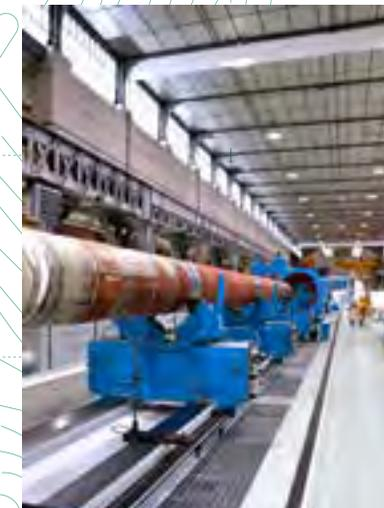
NAVAL GROUP IS INVESTING HEAVILY TO UPGRADE ITS INDUSTRIAL TOOL. AT ANGOULÊME-RUELLE, TWO NEW INDUSTRIAL MACHINING FACILITIES HAVE BEEN SET UP TO OPTIMISE THE MACHINING AND DRILLING CAPACITIES FOR THE SHAFT LINES, STRATEGIC COMPONENTS FOR THE SHIPS' PROPULSION SYSTEMS.
