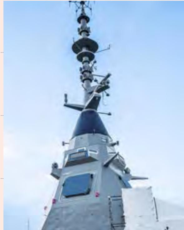
50 METRES HIGH AND WEIGHING 140 TONNES, THE PANORAMIC SENSORS AND INTELLIGENCE MODULE (PSIM) HOUSES A LARGE PART OF THE FDI COMBAT SYSTEM IN ITS UNIQUE MAST STRUCTURE.
